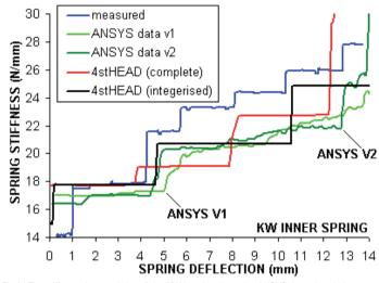
Fig.24 The stiffness characteristics of the 'KW inner' spring using ANSYS data v1 and v2.
