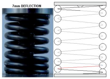
Fig.20 The 'KW inner' spring and its 4stHEAD model at 7 mm deflection.
