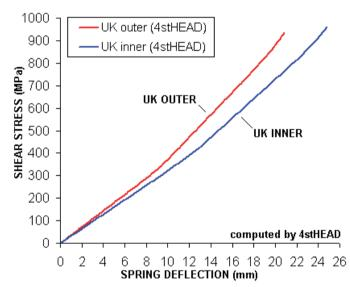
Fig.6 Computed shear stress characteristics of both UK springs.
