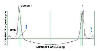
Fig.14 Matching measured valve jerk for racing design F.
